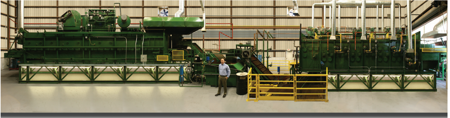
Peter Hushek and the automated, continuous cast link belt furnace that is used to process fasteners, stampings and screw machine parts. The furnace can handle 2,500 pounds an hour for either neutral or light case work.
