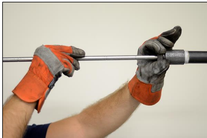
Figure 12 - Removing insertion rod from access port
