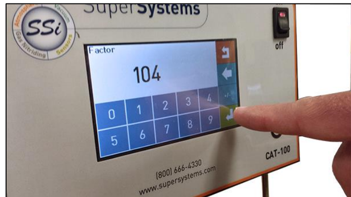
Figure 6 - Entering a new Coil Factor
