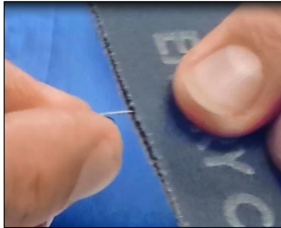
Figure 13 - Using emery cloth on wire coil
