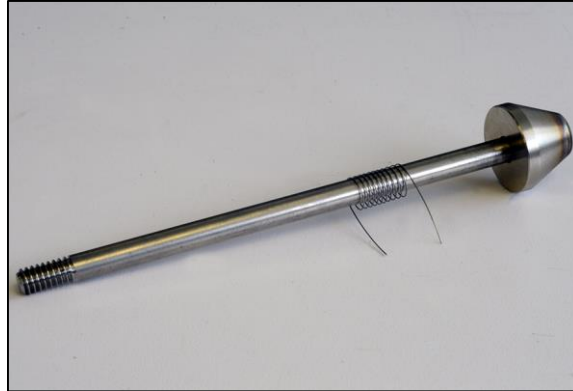
Figure 11 - Wire coil placed on rod screw
