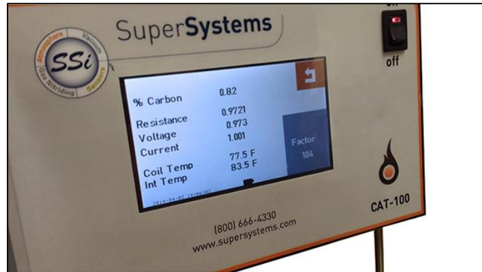
Figure 7 – Detail screen with new Coil Factor shown
